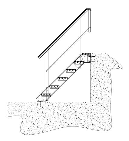
For fixing to adjecting structures GRP angle clips are used. See some details below.
