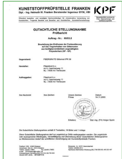
German 'Freibewitterungstest' for Fiberstruct IFR GRP gratings executed for the 44.000m 2 Wuppertal project
